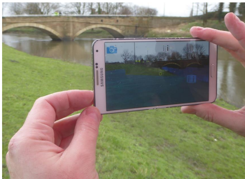
Fig. 4. Augmented Reality for visualization of flood levels. The blue plane displayed in the mobile phone shows the possible extent of the flooding. At the same time the white cube (i) allows the user to click and get real-time flooding information provided by a flood sensor.
